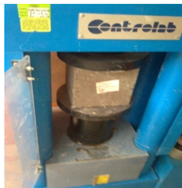
Figure 5.13: Essai de compression
