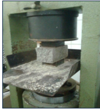
Figure 5.2 : Essai de compression
