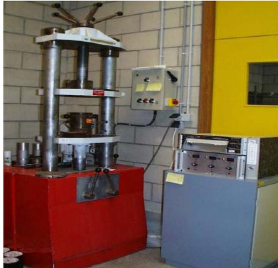
Figure (II-4) : Essai Duriez [16]
