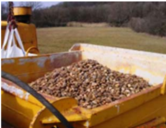
Figure 7-5 Ballast (gravier roulé 15/30 mm)
