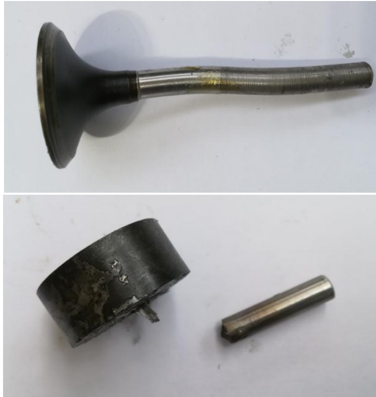
Figure 4-16- Endommagement du piston de compression.
