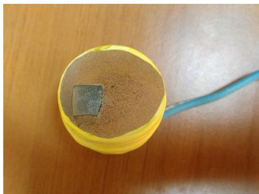
FIGURE 4.25:  chantillon 316L destin  au diff rents tests Versascan.
