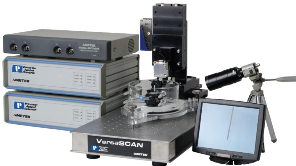
FIGURE 3.18: Station de balayage electrochimique Versascan.
