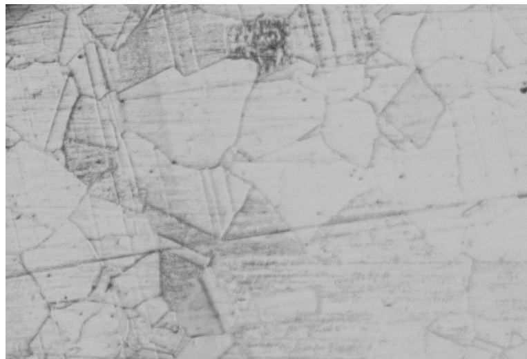
Figure 0.3 Microstructure la ZAT (x200).
