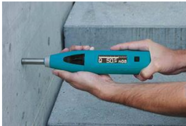
Figure II.5: Essai au marteau Schmidt.
