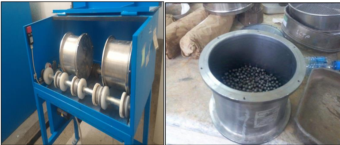
Figure 3.14. Machine Micro Deval [82].
