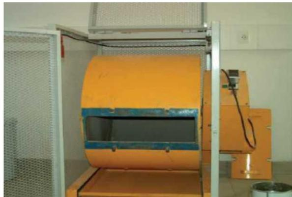
**Figure N°III-29:Essai Los Angeles**
