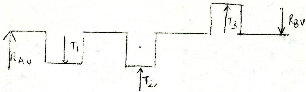
$$\sum \gamma_{\text{re}} = 0 \Rightarrow R_{AV} = \frac{T_1(l - l_1) - T_2(l - l_1 + l_2) - T_3l_3}{l}$$
