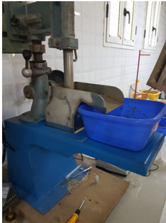
FIGURE 3.6: Cellule de flottation.
