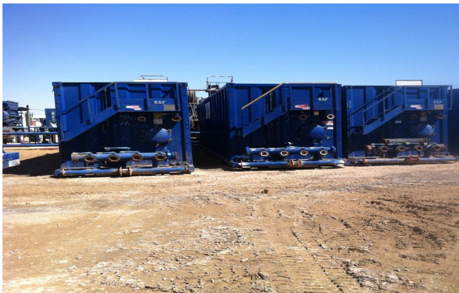
Figure 4 : Frac tanks (stage Schlumberger, 2015)
