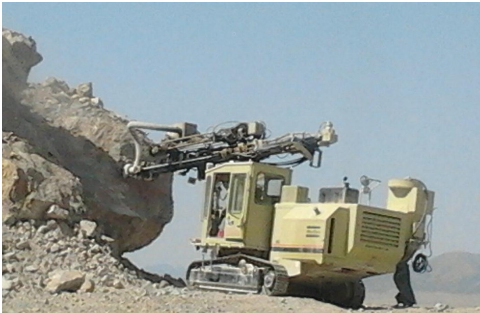
Figure III.4 : Chariot de foration
