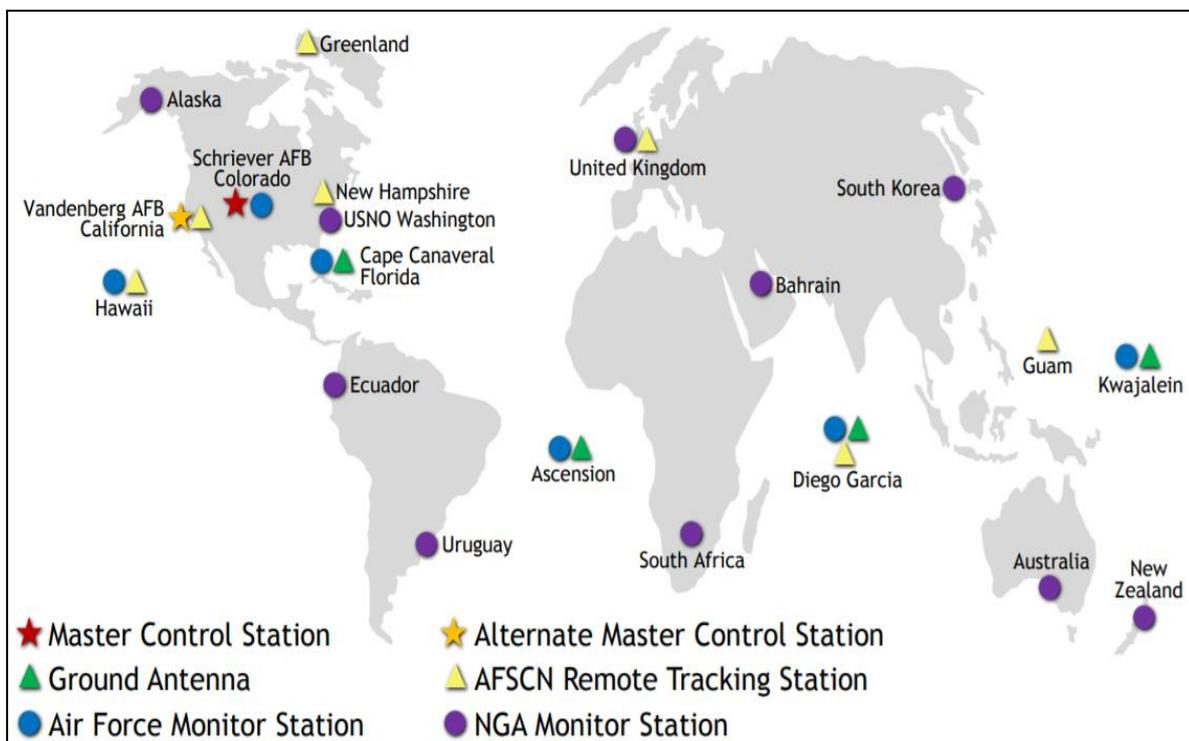
Figure 88. Le segment de control GPS [52]
