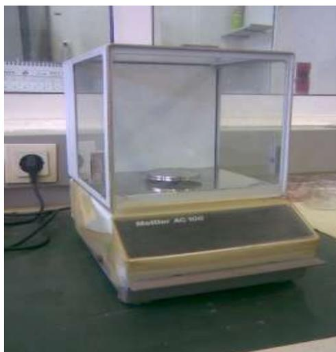
*Figure 11. Microbalance Mettler AC 1000.*
