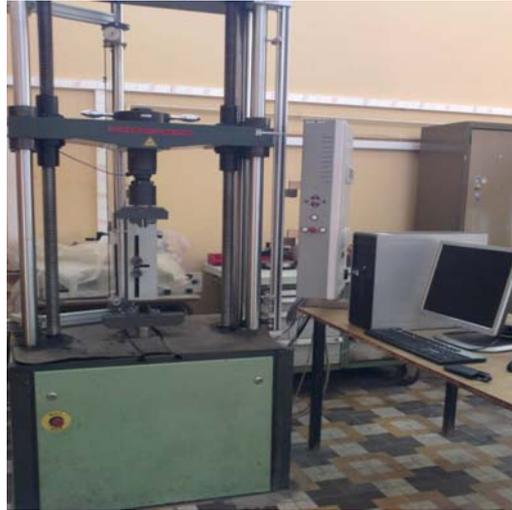
Figure III.25 : Machine de traction-compression " ZWICK/Roell"
