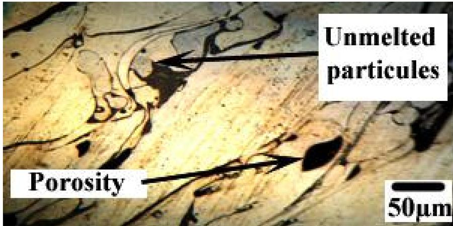
Figure 4. Micrography of thermanite (ASTM 301) coating.
