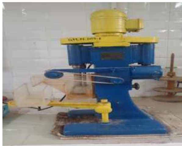
Figure III.7 : Cellule de flottation
