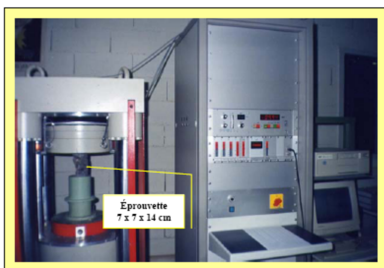
Fig. IX-7 – Presse hydraulique asservie (MOHR & FEDERHAFF Germany).
