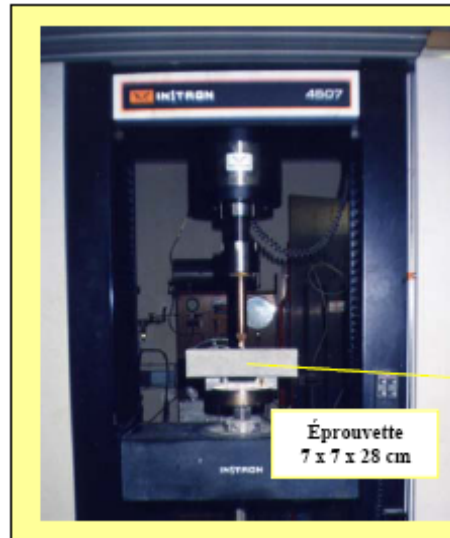
Fig. IX-9 – Machine universelle asservie (Instron 4507).
