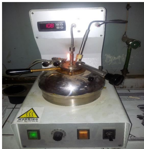
Figure 4.9 : Appareil PENSKY MARTENS
