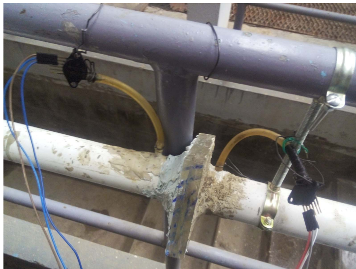
Figure 3.1: Using MPX4250AP to measure differential pressure.
