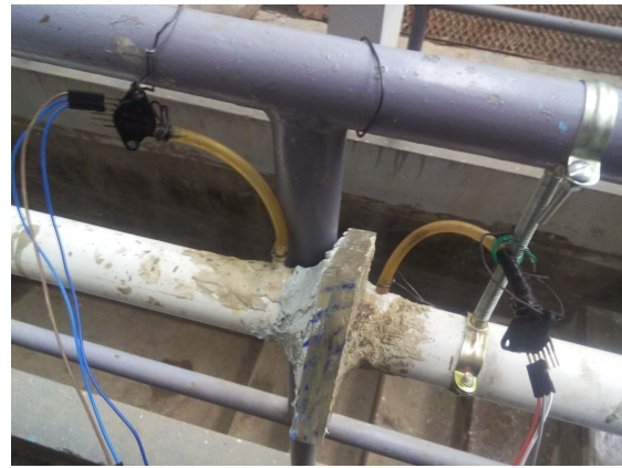
(a) The hydraulic system used to measure flow. (b) Measurement of differential pressure
