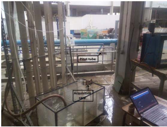
(a) The hydraulic system used to measure flow. (b) Measurement of differential pressure
