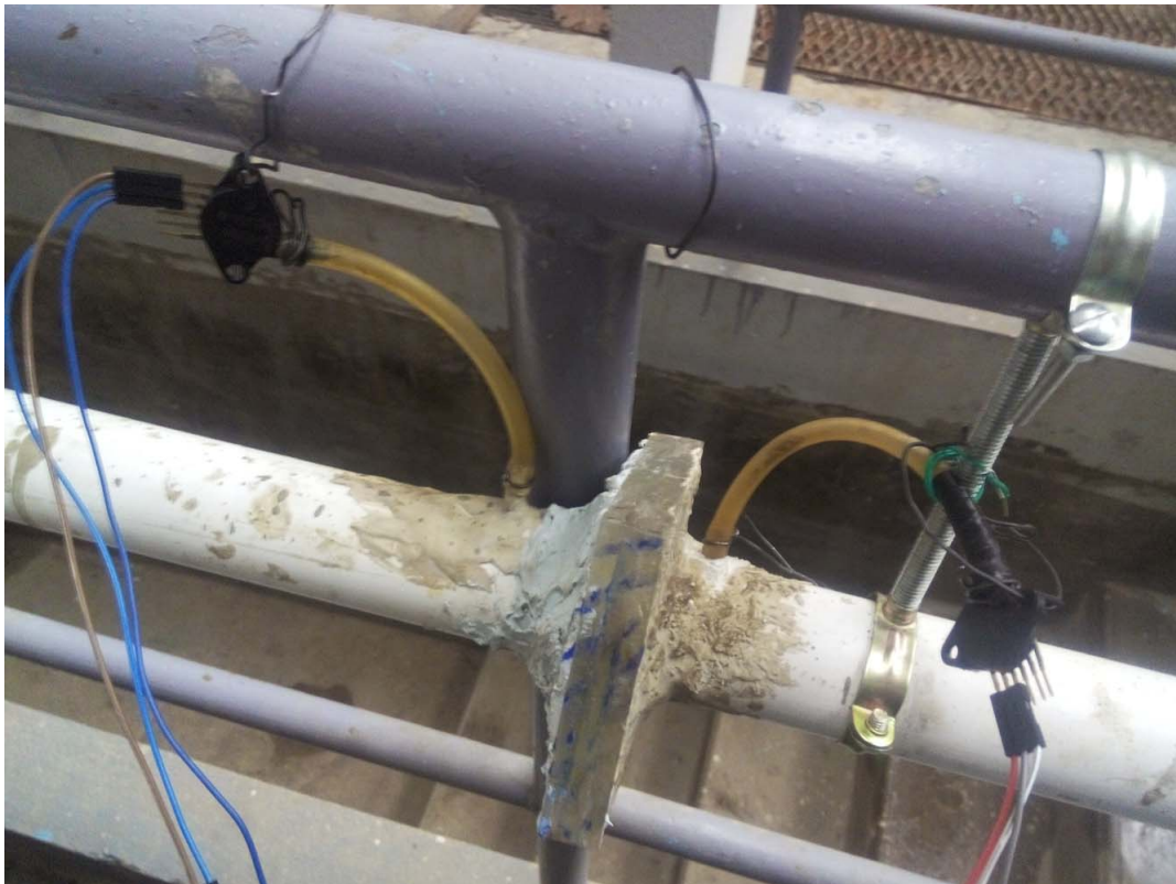
Figure 3.6: Flow measurement with two pressure sensors
