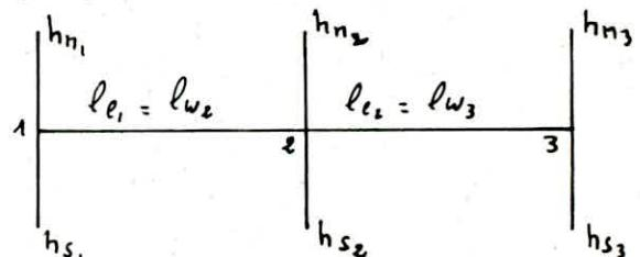
$$k_{e_1} = \frac{I_{e_1}}{l'_{e_1}} ; k_{s_1} = \frac{I_{s_1}}{h'_{s_1}} ; k_{n_1} = \frac{I_{n_1}}{h'_{n_1}} ; D_1 = k_{e_1} + k_{s_1} + k_{n_1}$$
