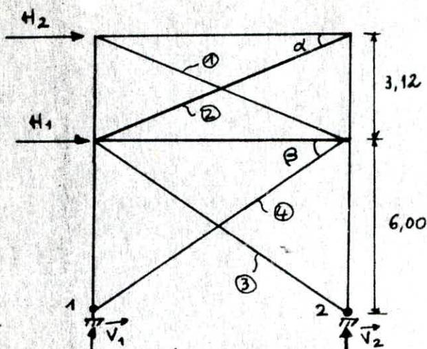
$$\begin{aligned} \tan \beta &= \frac{6}{6} = 1 \\ \rightarrow \beta &= 45^\circ \\ \tan \alpha &= \frac{3,12}{6} \\ \rightarrow \alpha &= 27,5^\circ \end{aligned}$$
