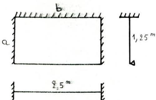
$$\left. \begin{array}{l} a = 1,25 \text{ m} \\ b = 2,5 \text{ m} \end{array} \right\} l = \frac{a}{b} = 0,5$$
