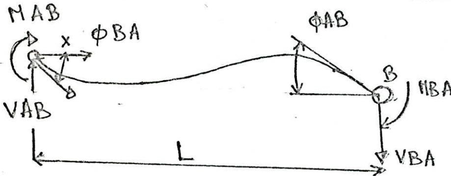
$$\text{on a } V_{AB} = V_{BA} = - \frac{(M_{AB} + M_{BA})}{L}$$
