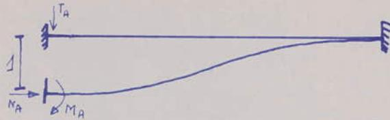
$$* \frac{\partial W}{\partial T_A} = \frac{T_A l_1^3}{3EI_1} - \frac{M_A l_1^2}{2EI_1} = 1 \quad (1)$$
