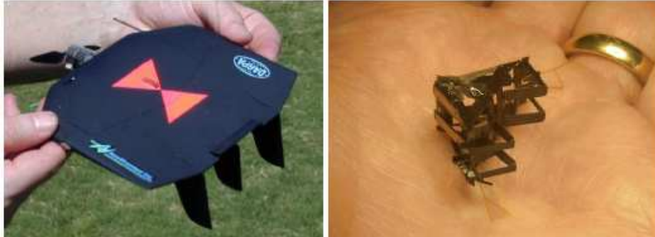
Figure 2.5: Micro drones: Black Widow (gauche) ET Micromechanical Flying Insect (UC Berkeley, 25mm).
