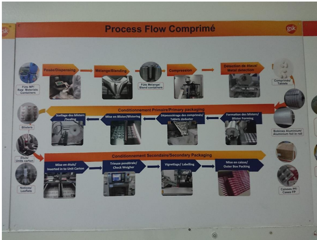
Figure 48 Processus de production Blister
