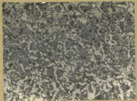
G = 400 O = 850 °C , Vr = 15°C/s Ferrite + Bainite + Martensite
