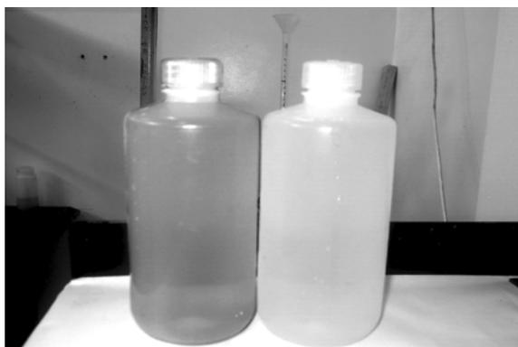
Fig. 2. Wastewater before and after electrocoagulation.
