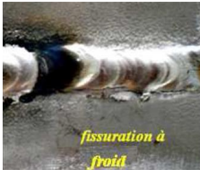
Figure III. 8: Fissuration à froid.
