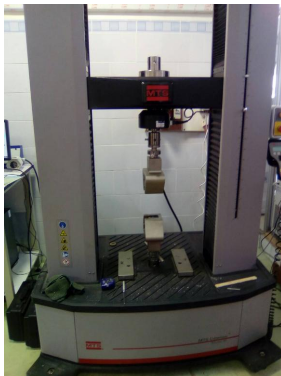
Figure 2.10 : Appareil de traction (MTS Criterion TM Model 45)
