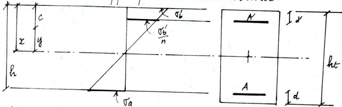
$$\text{on pose: } y = x - c \Rightarrow \frac{r_a}{n} = x - y + c$$
