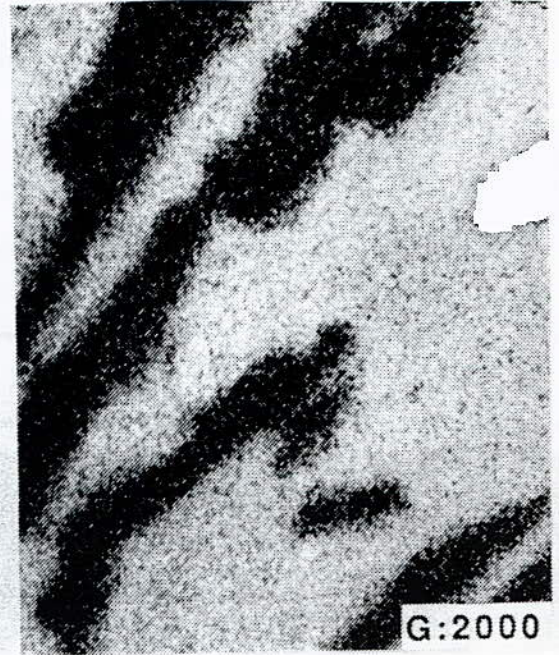
Figure II-18-b: Image X (SiK \alpha ) de la fonte M4B
