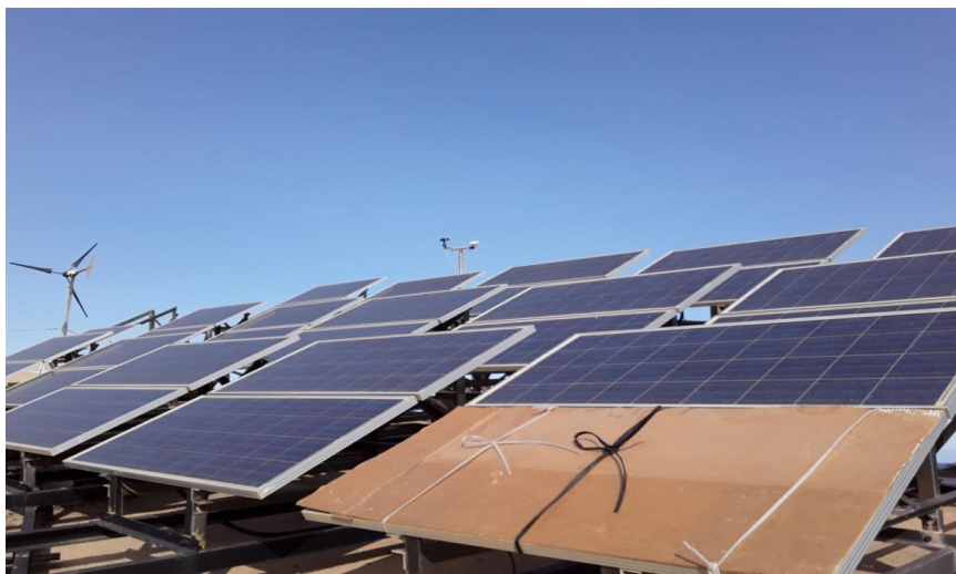
Figure 4.37 PV generator with one panel shaded of the SMS laboratory.
