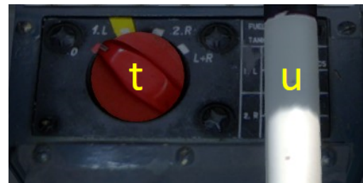
Figure 5.5 – Tank Switch et Flaps Switch
