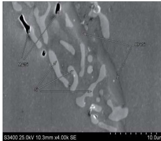
Figure II.5 : Morphologie des phases \alpha\text{-Al} + \beta\text{-AlFeSi} + \text{Mg}_2\text{Si} + \text{Si} [28]
